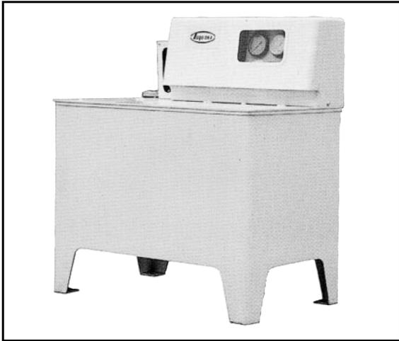
The hydraulic power unit is able to operate silently. This model has the pump directly coupled to the motor and the pump and motor assembly is immersed in the fluid in the reservoir. The result is drastic reduction of noise.
